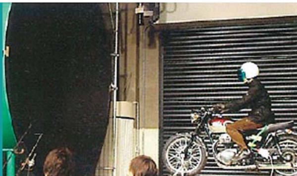
Wind tunnel experiment (Optimized Design Research and Development for Custom Parts based on Motorcycle Riding Posture Analysis via Ergonomics)
