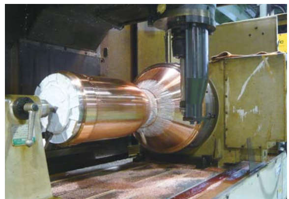
Machining of main nozzle for the engine for the H-IIA two-stage rocket
